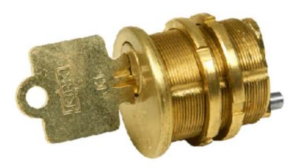
The Type CN22 (part# KC40---10) is a threaded cylinder interlock, commonly installed on circuit breaker interlocking kits. The cam on the back of the cylinder is made to interact with existing linkage on your equipment. The key is trapped or released according to the position of the cam. The CN22 can be linked to other CN22s with the proper bracketry.
