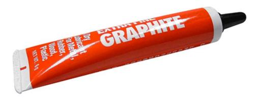
SD Series interlocks should be periodically lubricated with a small amount of dry powdered graphite. Do not use oil of any type as the oil will collect dirt and "gum up" the lock cylinder so that it will not operate.
