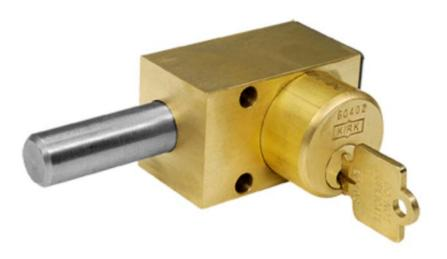
The Type NT interlock is similar in design to the Type F interlock. However, the Type NT housing is more narrow and is intended to be flat, or face mounted with 1/4" bolts through the front of the housing. It is ideal for applications where a smaller interlock or smaller mounting bolts are required for additional clearance (e.g. the front of a panelboard containing molded case circuit breakers).
