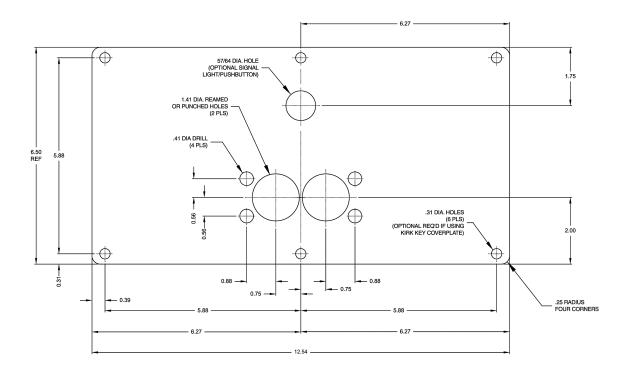
NOTE: This drawing provides the lock cylinder and mounting hole dimensions pertaining to unhoused Two-key SKRUs. It also provides overall dimensions and mounting hole locations for the cover plate if SKRU is purchased with cover plate only.
