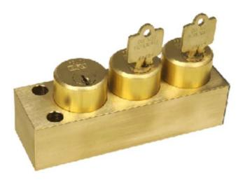
The Type T transfer block is an assembly of two or more lock cylinders in a single housing. Type T transfer blocks are designed to retain one or more keys (called held keys) while the remaining (initiating) key(s) are removed. This allows an exchange of keys for two or more interlock sequences. All initiating keys must be inserted into the Type T block before the retained keys can be removed. Once a retained key is removed, the initiating keys are trapped in the interlock.
